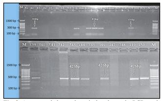
Fig. 8: Agarose gel electrophoresis that shown the PCR product determination of *sej* gene, Where M: marker 1500bp, agarose 1 %, TBE buffer (1x), 125 V with 25min Then 75 V with 1 hr and stained with ethidium bromide. Positive lane (Burn:B2.B6, B10-B12-B14, B19and Tonsils:T39, T42-T44, T46, T49, T50) N: negative control and visualized on a UV transilluminat or documentation system.
